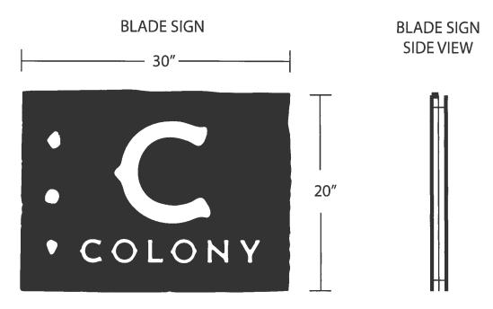
Water jet cut 14 gauge plate steel - doublesided Matte black powder coat finish Lettering and graphics elements white matte acrylic panel sandwiched between steel panels with 1/4" standoffs between layers Fastened to building using c-channel blade bracket
