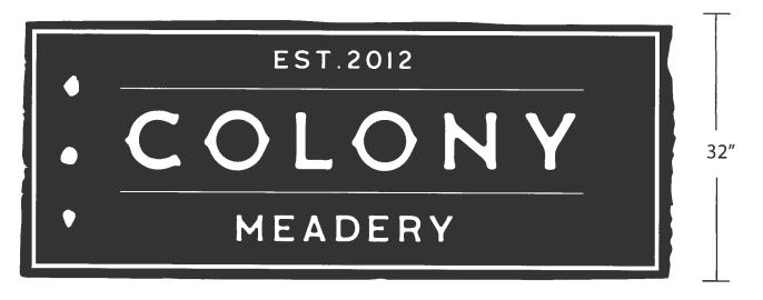
Water jet cut 14 gauge plate steel Matte black powder coat finish Lettering and graphics elements semi-translucent white matte acrylic backer panel Back-lit with led contained within 2" depth aluminium box Blind fastened to building through light box and hidden brackets
